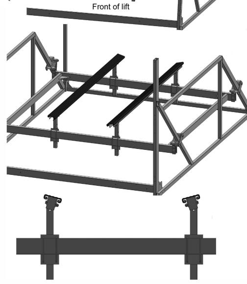
Tighten all the bolts. Put boat on lift and check for clearances. Pull the boat off the lift and adjust as needed. The boat should be around a foot off the back of the lift and 1" above the bed.
