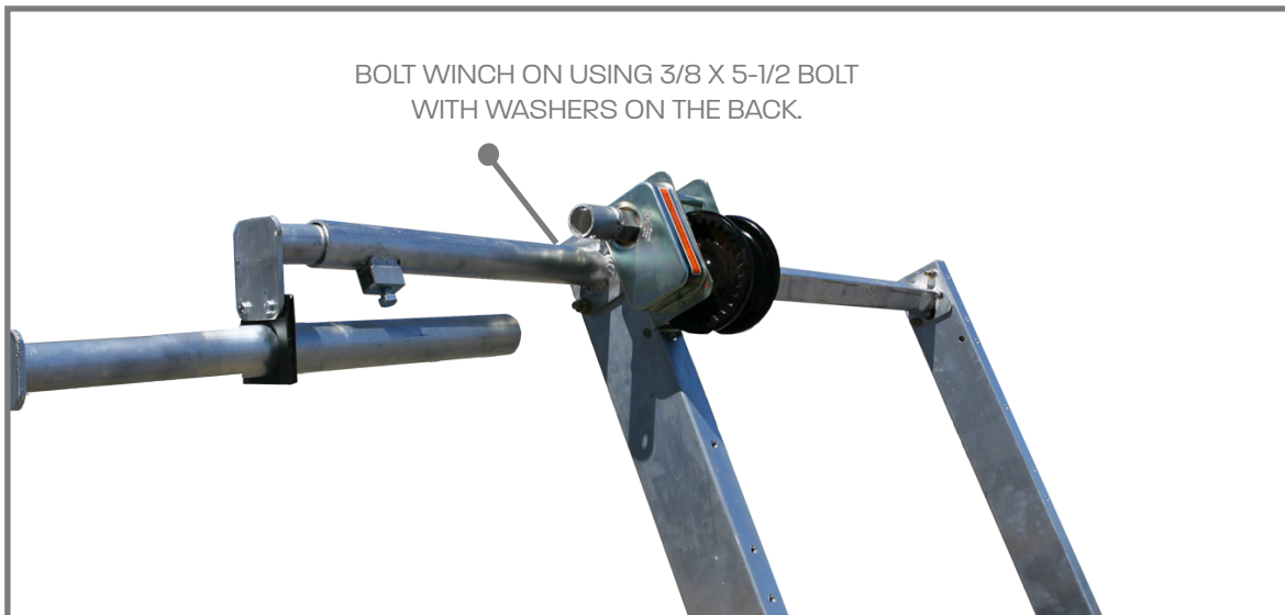
(2) 3/8 X 5-1/2 BOLT WITH WASHERS & NUT ON THE BACK TO HOLD THE WINCH ON.
